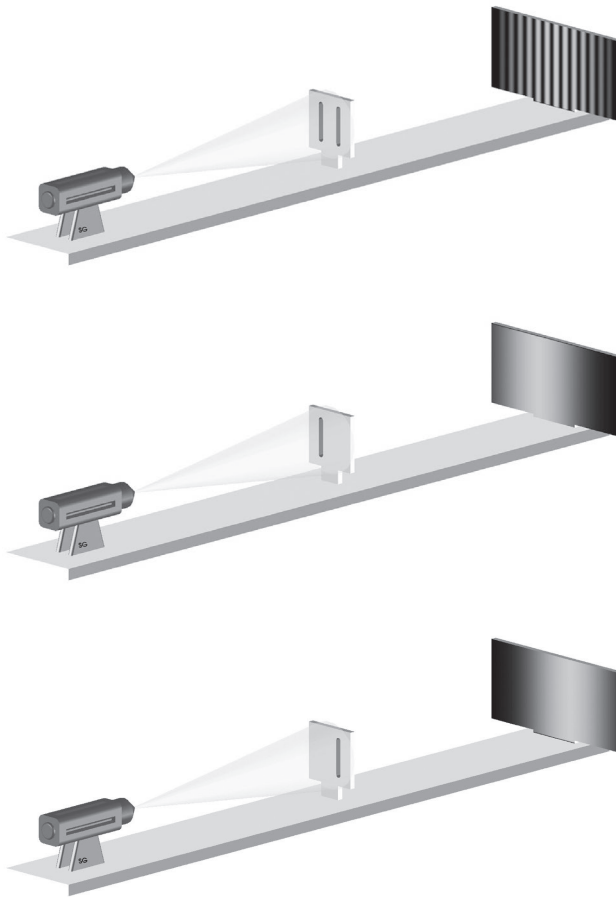
Figure 2. Thomas Young's double-slit experiment in a modern version. The light emitted by a laser passes through two slit openings in a diaphragm. Finally, it hits an observation screen. When both slits are open ( top ), we see a series of dark and bright stripes, called "interference fringes." If only one of the two slits is open ( middle and bottom ), we observe a broad illuminated area without any stripes. It is clear that the striped pattern in the top picture, when both slits are open, is not the sum of the two others. Rather, at the dark locations, the two waves coming there from the two slits extinguish each other. At the bright locations, they reinforce each other. The extinction at the dark stripes and the amplification in the bright stripes are a clear confirmation of the wave nature of light.
